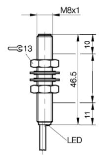
Inductive Sensors BES 516-378-EO-C-02 M8x1 x 46.5 normally-closed Sn=1,5mm shielded
